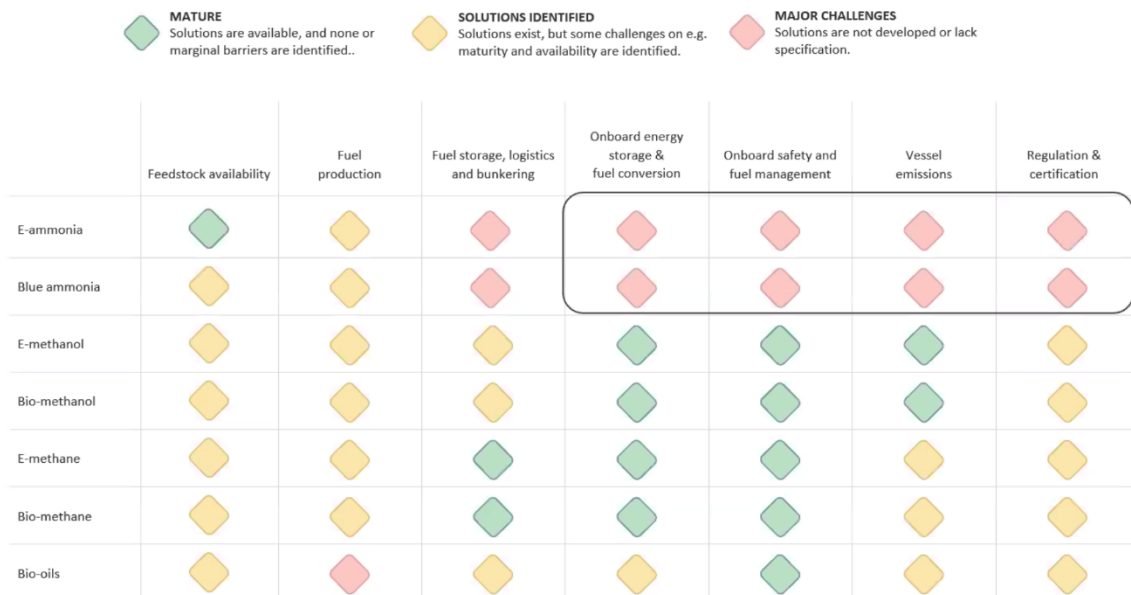
Fig.1 Maturity of alternative fuels according to https://www.zerocarbonsshipping.com , Thomas McKenney at “Ammonia for shipping” webinar Dec. 12, 2022. The project looks at intercontinental shipping, hence batteries not on the list.
